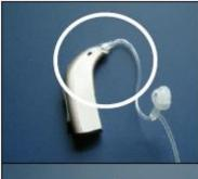
**Step 1:** Disconnect the tubing at the top where it joins the hearing aid.
