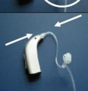
Step 4: Reconnect the tube to the hearing aid by firmly pushing the top of the tube back into the opening. Lightly tug the tube to ensure that it is connected securely.
