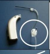
**Step 3:** Feed the wire all the way through the tubing to clear any wax/debris.
